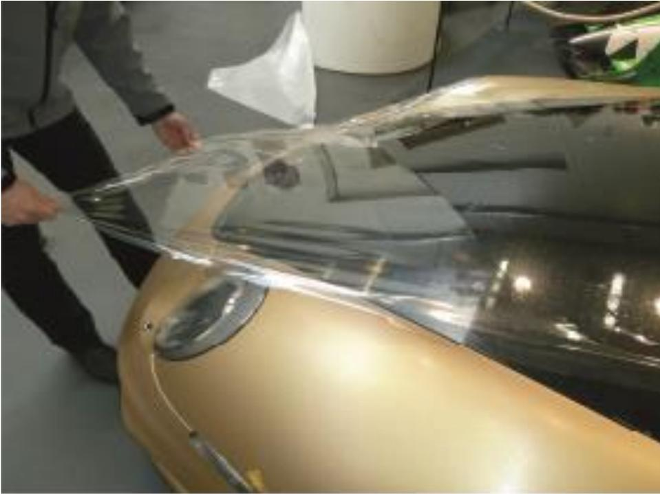
These films are meant to protect the vulnerable parts of cars, bicycles, motorbikes, etc...
