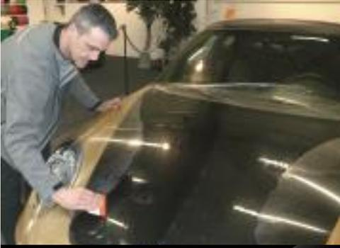
9. Start rubbing in the middle of the vinyl. Also rub towards the closest edge, making sure that the slip solution mixture can always be rubbed to the sides. Avoid air- and/or water bubbles. It is hard to puncture them afterwards.
