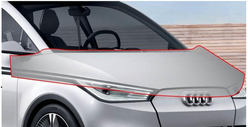
In case of wet wrapping, the chance of air bubbles getting entrapped or rubbing stripes appearing in the glue becomes a lot smaller. However, this method is only advisable if the part to be wrapped does not or hardly show any deformation. It will also take longer for the film to reach its final adhesive strength.
