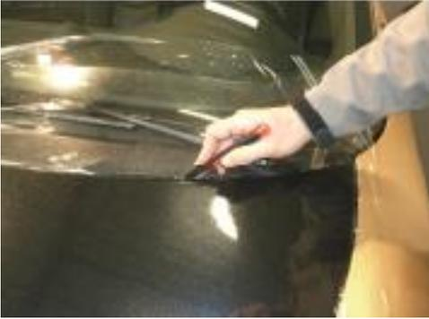
13. All excess material can be cut off with a very sharp knife. You can also use a razor blade for this job. Afterwards fold the vinyl around the edges. This will make the edges of the vinyl on the car body invisible.
